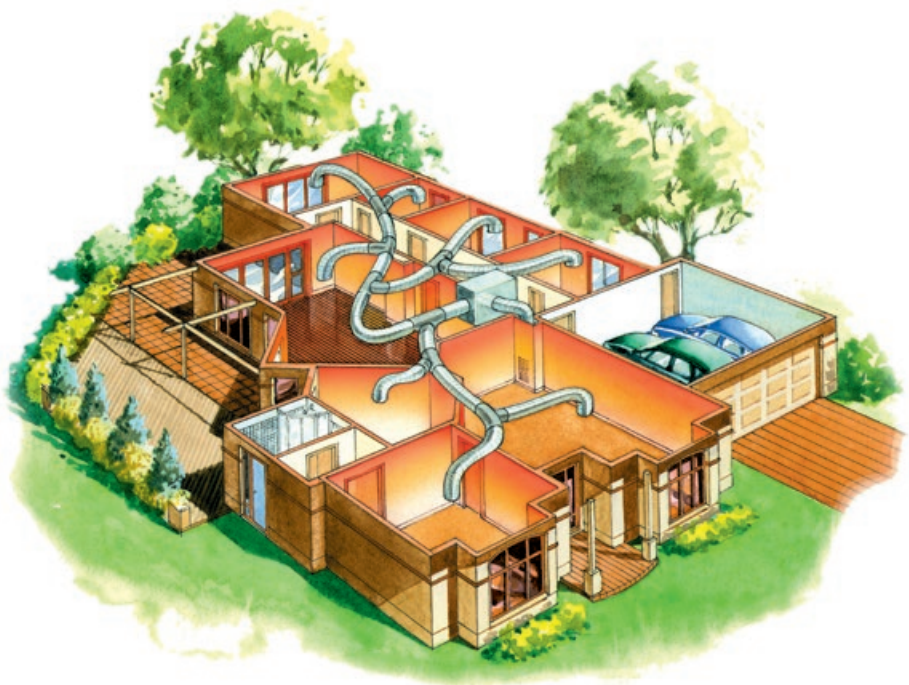
Typical unit and ducting layout of a Bonaire Ducted Heating System (internal unit installation)
